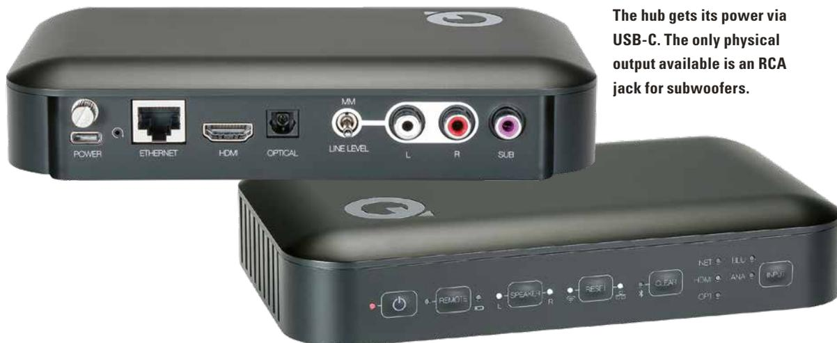
The hub gets its power via USB-C. The only physical output available is an RCA jack for subwoofers.
